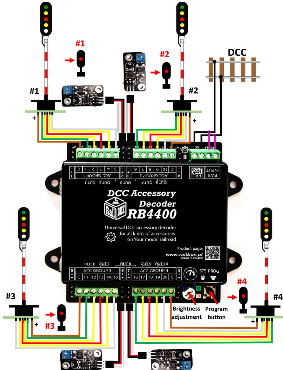
The signal S1 trigger PCB acts as a track occupancy sensor, after driving train from Track section 1 (place the semaphore here) to track section 2 (Connect the sensor in between), the red signal (S1) will be automatically turned on. Connecting the S1 signal trigger to the tracks:
